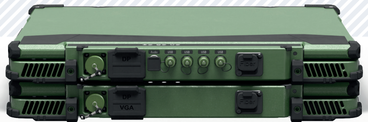
Interfaces protected from the elements (rear view of variant SDIP 27 Level A (top), Zone 1 (bottom))
